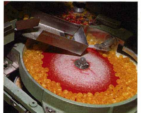
The wrapping room is held below 45% relative humidity so candy dust does not stick and clog machinery. Storing the wrapping material in the dry room allows high speed wrapping, even when using polypropylene.
