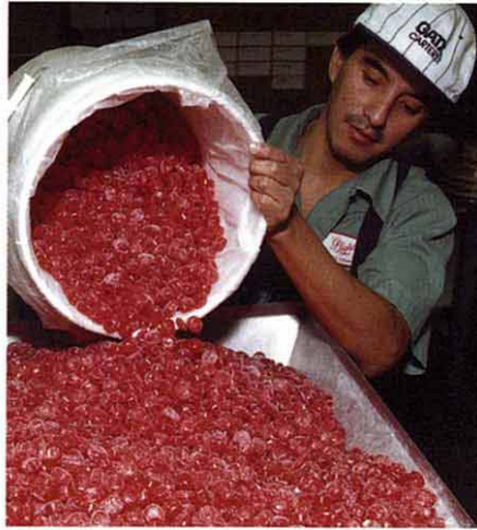
Controlling humidity below 45% relative humidity in the bagging room reduces friction between candy pieces, which prevents "bridging" and avoids the lost profits of overweight bags.
